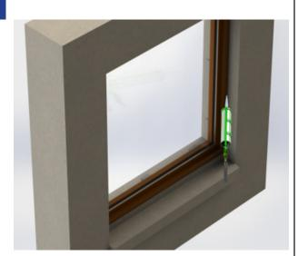
If total frame replacement in brick or siding was preformed maintain a minimum of 3/8" between the window frame, trim, siding, or masonry. Failure to do so could cause product or property damage.
