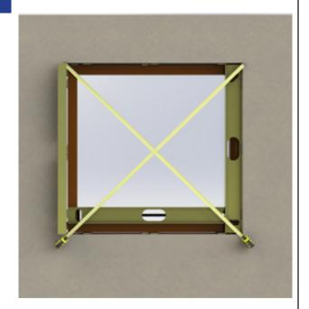
Place a level on the window sill to verify that the sill is level. Adjust the shims as needed to ensure a level condition. Check the head, sill and jambs with a level again to make sure the window is setting plumb, level, and square within the opening. Measure across the diagonals to determine if the window is square.
