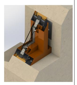
Operate window unit to ensure proper operation. Sash will not operate correctly if window is out of square, overshimmed or over-insulated.
